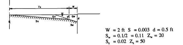
Calculate  $Q_w$  by subtracting the Q's at depth d based on an extension of slope ratio  $Z_w$  to intersect the water surface and at a depth d', where d' = d - W/Z<sub>w</sub>, thus  $Q_w = Q_d - Q_d'$ . Calculate  $Q_s$  for a slope ratio of  $Z_s$  and depth d'. Then  $Q = Q_w + Q_s$ .
