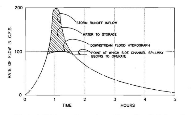
Effect of Offstream Reservoir on Storm Runoff Hydograph
