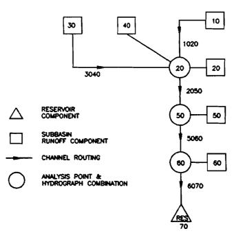
Figure 2-29 Example Drainage Basin Schematic
