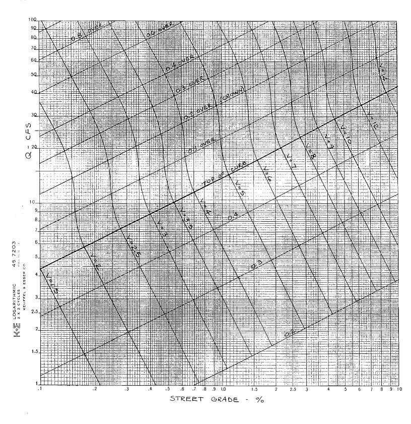
FLOW CAPACITY V2 STREET SECTION 45' B-B
